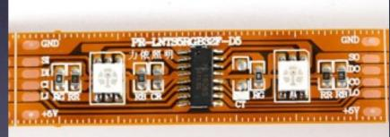
RGB LEDs chained together with shift registers transmit info down the strip and light up according to instructions from Arduino
