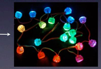
RGB LEDs chained together with shift registers transmit info down the strand and light up according to instructions from Arduino (intrinsic PWM)
