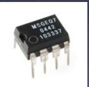
Uses frequency info to send pattern commands to LED strips
