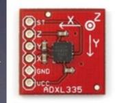
Accelerometer gives measure of 3D motion
