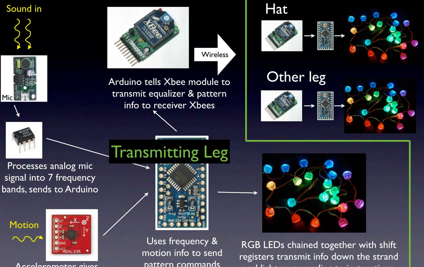
Accelerometer gives measure of 3D motion pattern commands to LED strands
